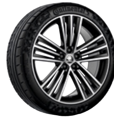
Sirius 654 071 498G FL8 light-alloy wheel 7.0J x 18" ET39 for 205/45 R18 black metallic brushed
