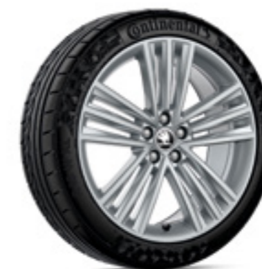
Sirius 654 071 498M 8Z8 light-alloy wheel 7.0J x 18" ET39 for 205/45 R18 silver metallic
