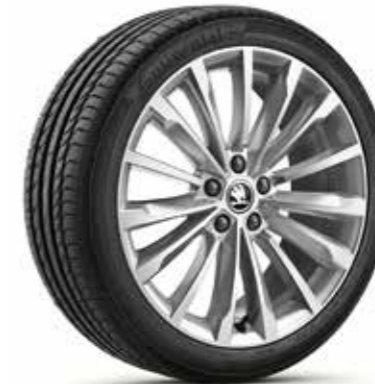
Trinity 3V0 071 499E 8Z8 light-alloy wheel 8.0J x 19" for 235/40 R19 tyres ET44, silver metallic brushed ŠKODA Genuine Accessories
