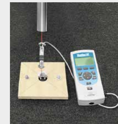
Testing of fixing element strength
