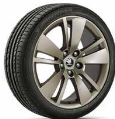
Zenith 3VO 071 498D HZ9 light-alloy wheel 8.0J x 18" for 235/45 R18 tyres ET44, platinum matt ŠKODA Genuine Accessories
